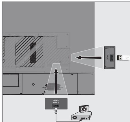
1 Connect the **USB 2 (HDD)** USB interface on the television and the related data output on the external device (external hard disk, digital camera, card reader or MP3 player) with a USB cable;
