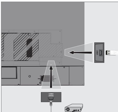
1 Plug the external hard disk to the **USB 2 (HDD)** USB interface of the television;
